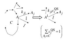
Fig. 5. Gluing a cycle with rate constants renormalization.  $c_l^{\rm QS}$  are the quasistationary concentrations on the cycle. After gluing, we have to leave the outgoing from  $A^1$  reaction with the maximal renormalized rate constant, and delete others.
