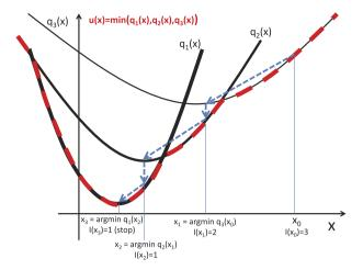
**Fig. 2.** Optimization of a one-dimensional minorant function u(x), defined by three functions  $q_1(x)$ ,  $q_2(x)$ ,  $q_3(x)$  each of which has a local minimum. Each optimization step consists in determining which  $q_{I(x)}(x) = u(x)$  and making a step into the local minimum of  $q_{I(x)}$ .
