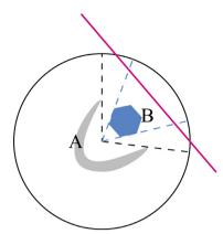
Fig. 4. Linear separability via projection onto a sphere. Sets A (shown as a shaded gray domain) and B (depicted as a blue filled hexagon) are not linearly separable in the original coordinates. Their projections onto the sphere, however, are separable (the separating hyperplane is shown in red). (For interpretation of the references to colour in this figure legend, the reader is referred to the web version of this article.)
