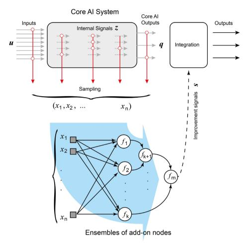
Fig. 1. Functional diagram of correcting neuronal ensembles for a generic Artificial Intelligence system.
