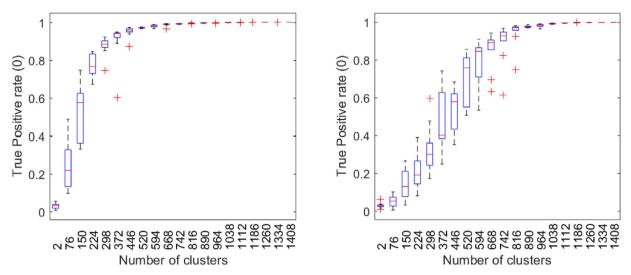
**Fig. 9.** True Positive rate at  $\gamma = 0$  for the combined system as a function of the number of clusters, p. Left panel corresponds to Algorithm 1 with the optional projection step. Right panel corresponds to Algorithm 1 without the projection step.
