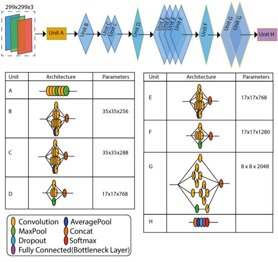
Fig. 5. Architecture of the adopted Inception deep neural network model. (For interpretation of the references to colour in this figure legend, the reader is referred to the web version of this article.)
