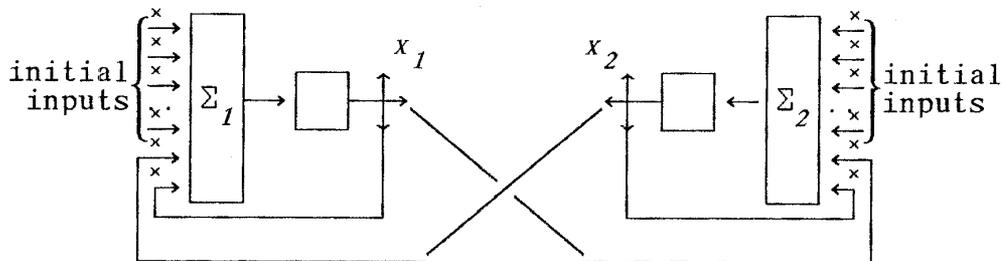
Fig. 1. Layout of the two-neuron expert. The symbol  $\times$  shows that the input signals are multiplied with the input's weights.
