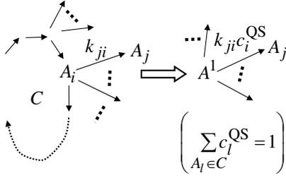
Fig. 5. Gluing a cycle with rate constants renormalization.  $c_i^{\text{QS}}$  are the quasistationary concentrations on the cycle. After gluing, we have to leave the outgoing from  $A^1$  reaction with the maximal renormalized rate constant, and delete others.
