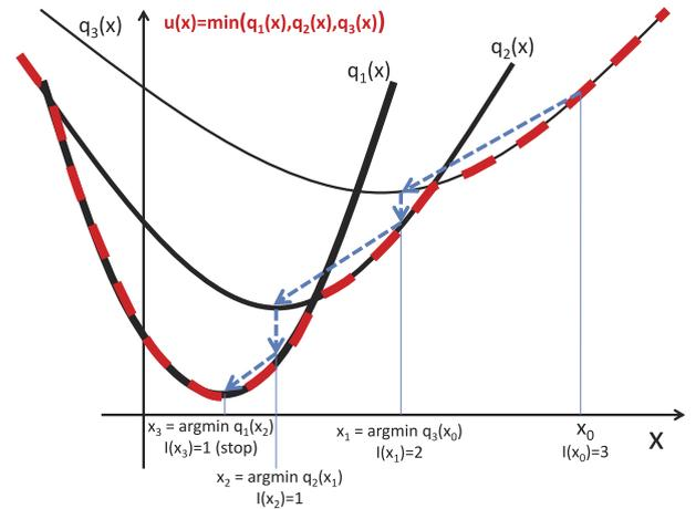
**Fig. 2.** Optimization of a one-dimensional minorant function  $u(x)$ , defined by three functions  $q_1(x), q_2(x), q_3(x)$  each of which has a local minimum. Each optimization step consists in determining which  $q_{l(x)}(x) = u(x)$  and making a step into the local minimum of  $q_{l(x)}$ .
