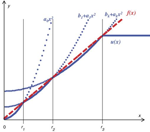
**Fig. 1.** Trimmed piecewise quadratic potential of subquadratic growth  $u(x)$  (solid blue line) defined for the majorating function  $f(x)$  (red dashed line) and several thresholds  $r_k$ . Dotted lines show the parabolas which fragments are used to construct  $u(x)$ . The last parabola is flat ( $a_p = 0$ ) which corresponds to trimmed potential. (For interpretation of the references to color in this figure legend, the reader is referred to the web version of this article.)
