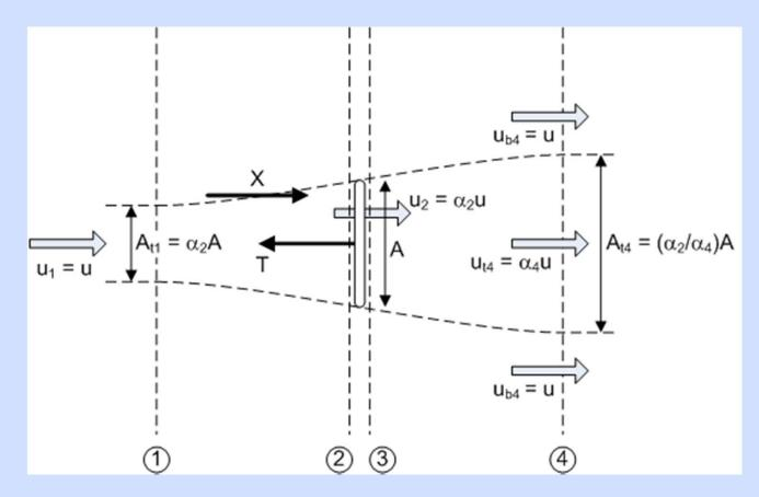
For **wind turbine** in free air, mass/momentum analysis shows that stream tube area increases and velocity decreases through the turbine.
