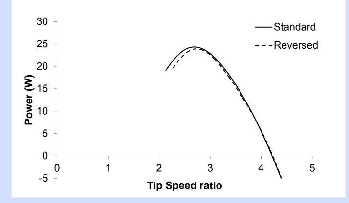
Truss device tested in standard and reversed configurations at Fr = 0.18
