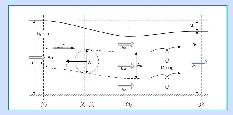
Power extracted from turbine best represented by Head efficiency
