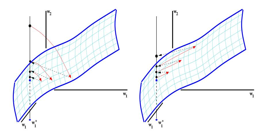
The relative orientation of the slow manifold and the fast fibers affects algorithm convergence
