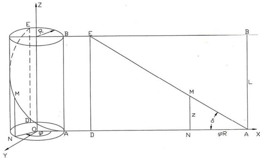
**Figure 7. Isometric projection of blade line EMA on vertical plane**
