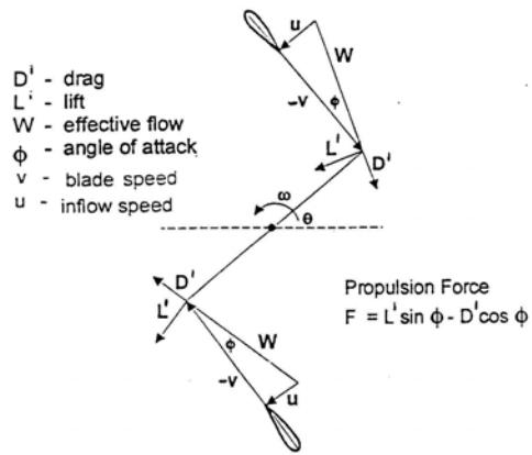
**Figure 6. Double-Helix Turbine Diagram**
