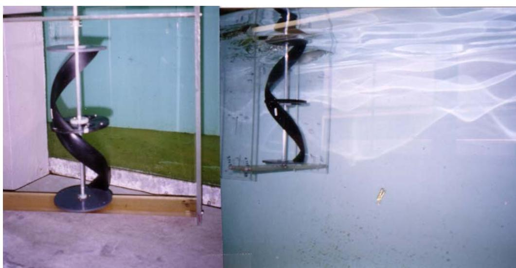
**Figure 5. Single Helix Turbine tested at Northeastern University
